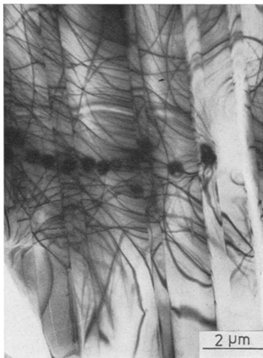
Figure 6 Hornblende lamellae in grunerite. The contamination spots were produced during analysis with EMMA-4.
